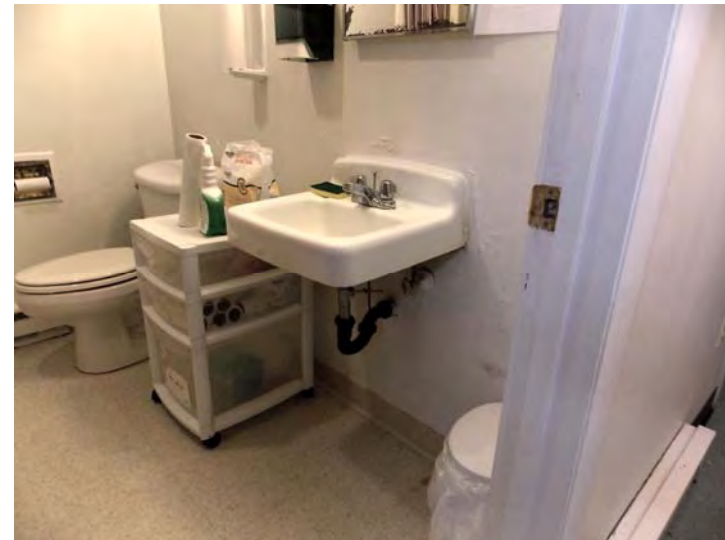
The standard bathroom has a wall-hung sink, VCT flooring and a low flush toilet.
